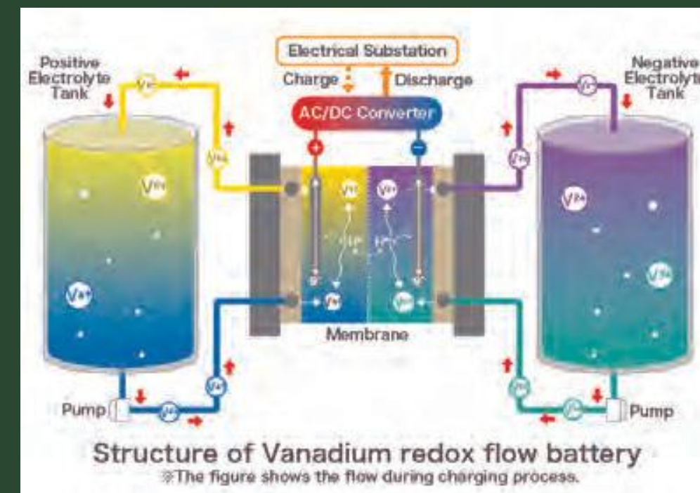
Vanadium Redox Flow Batteries (VRFBs)
